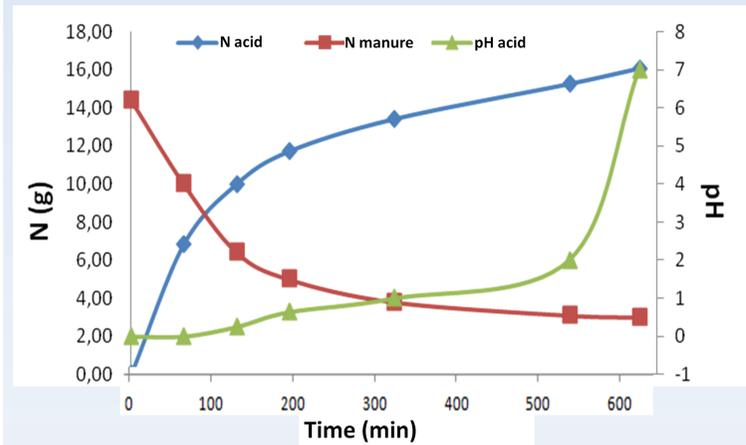
Membrane developed has shown good performance when treating **synthetic input flows** **87% of NH<sub>3</sub> recovery** was achieved.
